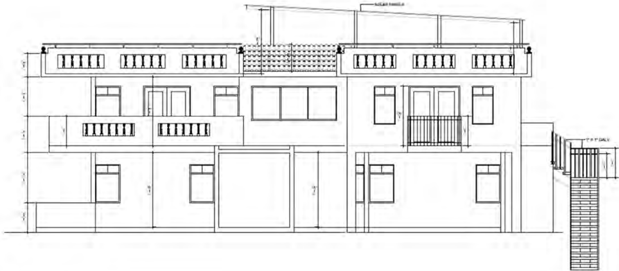
NEW FRONT ELEVATION SCALE: 1/4" = 1'-0"
